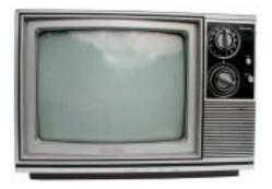
copper wire (one percent), engineering plastics (seven percent high-impact polystyrene), and low-grade circuit boards (ten percent), which all represent revenue to the recycler. The large volume of waste is attributed to old wood consoles, laminated plastic housings and other plastic housings contaminated with paint and/or metal that were common in the 1970s and 1980s.
